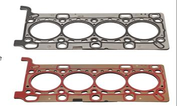
In addition, the connection between the individual metal layers has been changed. The gasket with item number 598.670, which is no longer produced, was connected with four weld spots. On the successor gasket, item number 867.700, the metal layers are now permanently connected to each other with rivets. This does not essentially change anything in terms of the installation of the cylinder head gasket.
